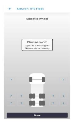
After scanning the gateway ID, you will see a countdown menu of 120 seconds. This is to ensure that all sensors on the vehicle are instructed to go into Tap & Tell mode. Wait until the countdown is complete.
