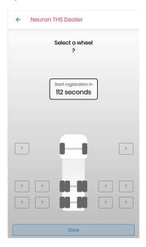
When the countdown is finished you mark the tyre you want to register in the app and knock twice with a hammer. The two knocks need to be within a second to be registered. Observe that the changes to before you move on to the next tyre. This will happen within a second, if not, repeat the two knocks.
