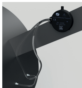
Keep antenna clear off the metallic surface
