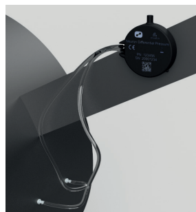
Keep antenna clear off the metallic surface
